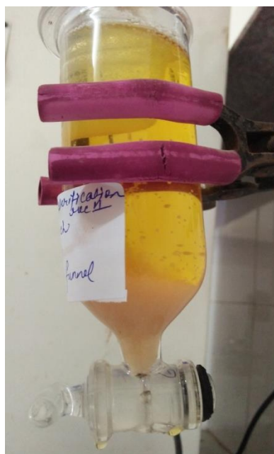
Figure 3. Clear separation of methyl ester and glycerin observed after transesterification reaction.
