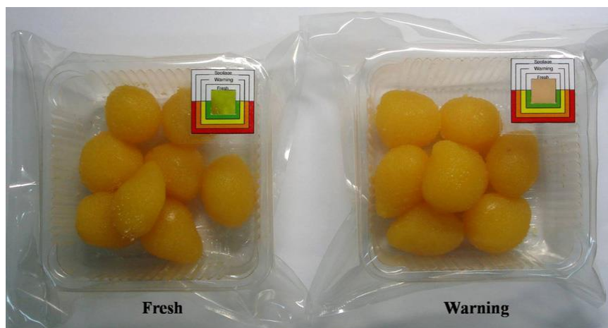
Figure 15. Packaged Golden Drop with Food Spoilage Indicator Label (Green = Fresh; Orange = Warning) [44].
