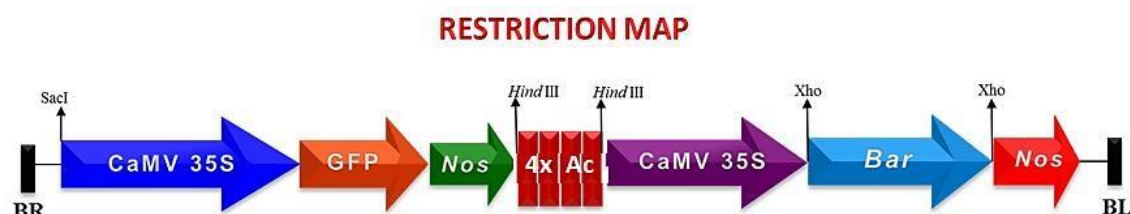
Figure 4. This figure represents T-DNA construct by harbouring different expression units and it is named as pSB111-Bar-4XAc-GFP vector and it shows the restriction map of Hind III, SacI and xhoI restriction enzymes.
