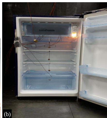
Figure 4. Thermocouples attached at different compartments for ice-making and pull-down test
