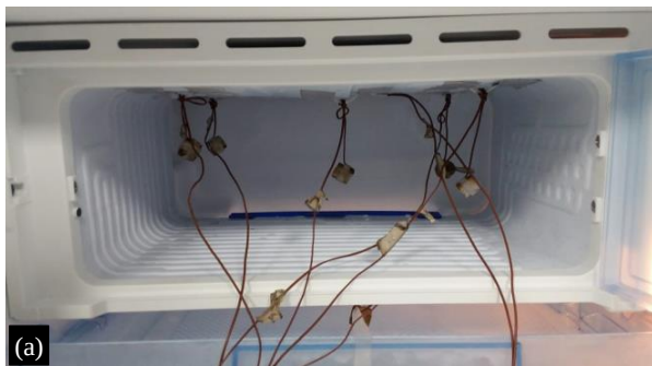
Figure 4. Thermocouples attached at different compartments for ice-making and pull-down test
