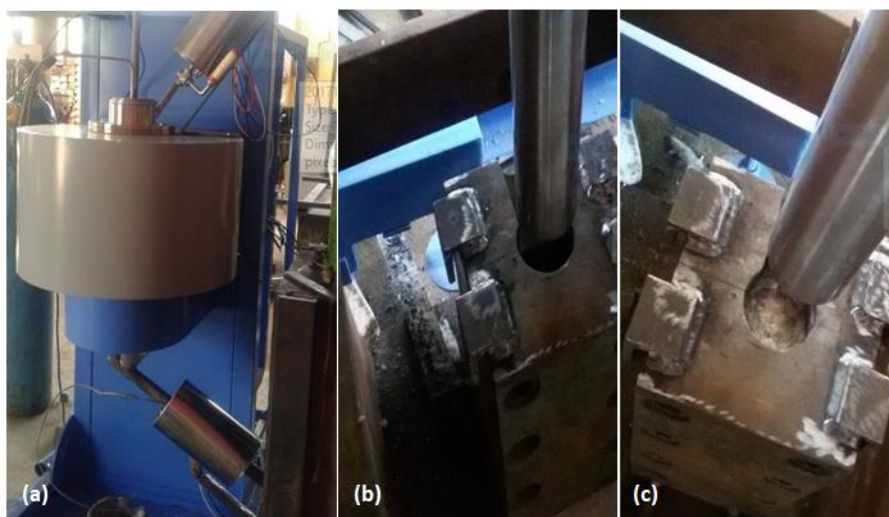
Figure 1. Sequential diagrams representing fabrication of (a) squeezed stir casting machine, (b) squeezed pressure setup before pouring, and (c) squeezed pressure setup after pouring the AZ91-melt.
