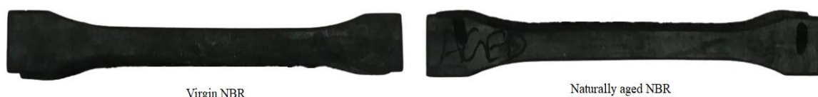
Figure 3. Dog-bone Specimens of NBR.
