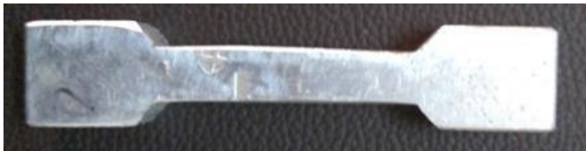
Figure 1. Developed nano-carbon-doped aluminium oxide sample as per ASTM D 638-03 size.
