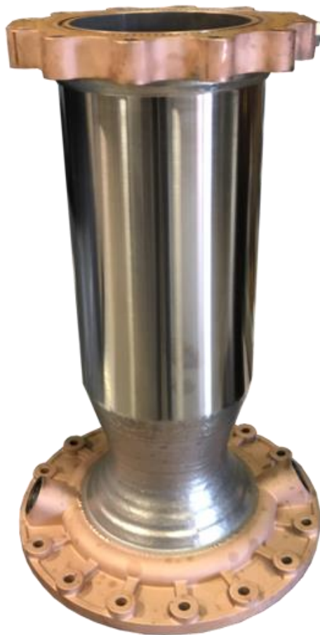
Figure 5. 3D-printed bimetallic lightweight thrust chamber assembly before hot-fire testing at NASA's Marshall Space Flight Center in Huntsville, Alabama [Image credit: NASA].
