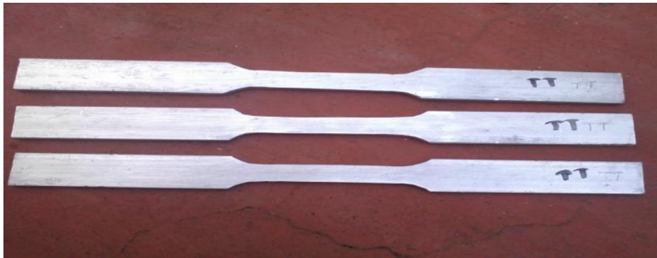
Figure 2. Aluminum alloy 6063 tensile test specimen without damage.
