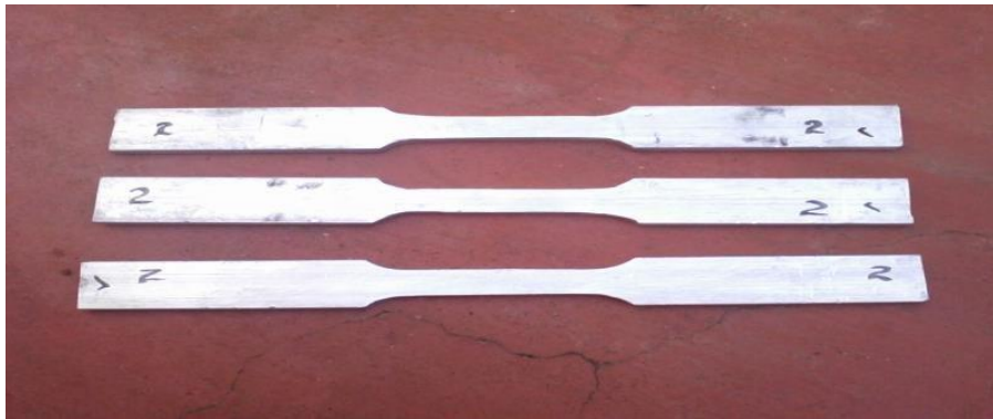
Figure 4. Aluminum alloy 6063 tensile test specimen with 2J damage.
