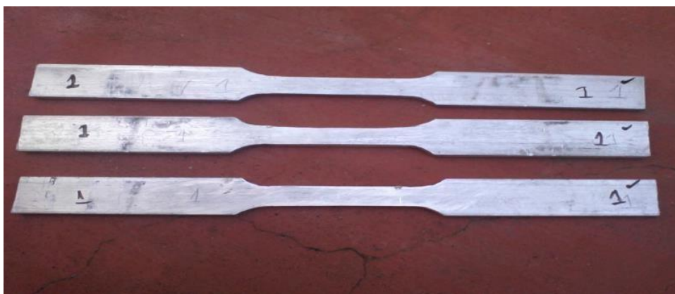
Figure 3. Aluminum alloy 6063 tensile test specimen with 1J damage.
