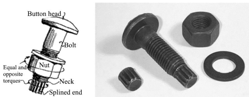
Figure 3. Typical tension controlled bolt [7].
