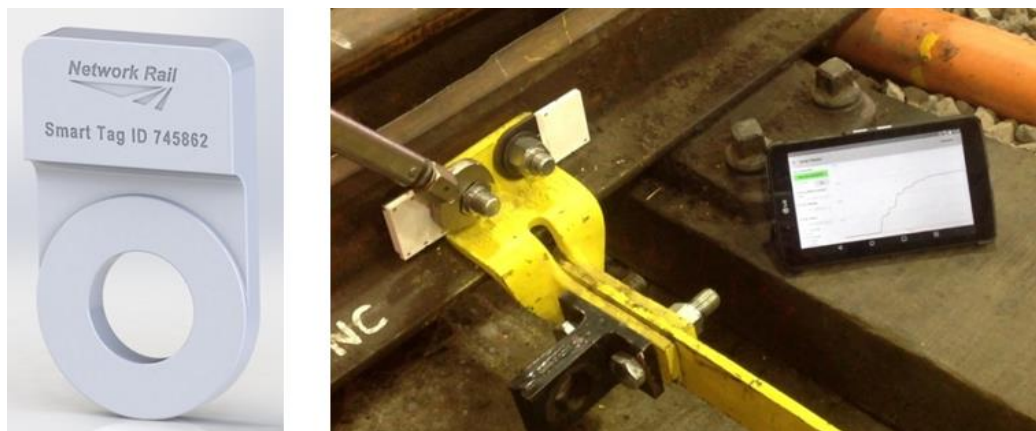
Figure 8. Smart washer and data reading unit [20].
