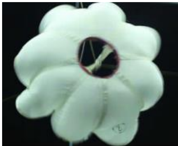
Figure 4. Wind tunnel test photograph of parachute.
